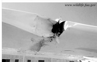
Bird impact traces on aircraft's nose/wing
