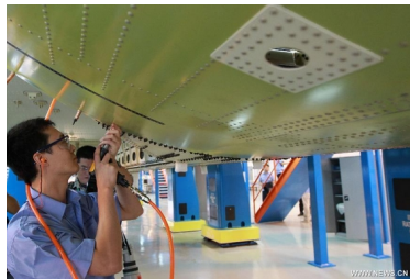
Fuselage of modern aircraft contains \approx 100\,000 rivets
