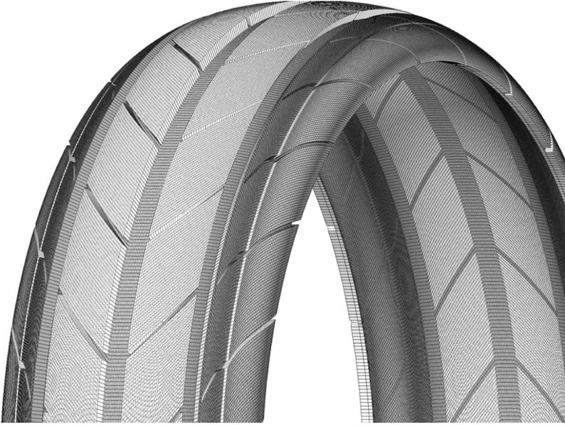
**Fig. 8** A part of the tyre finite element mesh consisting of about 550,000 nodes.
