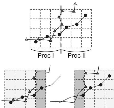
constructed contact elements between the corresponding subdomains. If a contact element unions slave node and master nodes from different subdomains, the interface between them has to be created or updated as well as duplicated slave or master nodes have to be formed.
