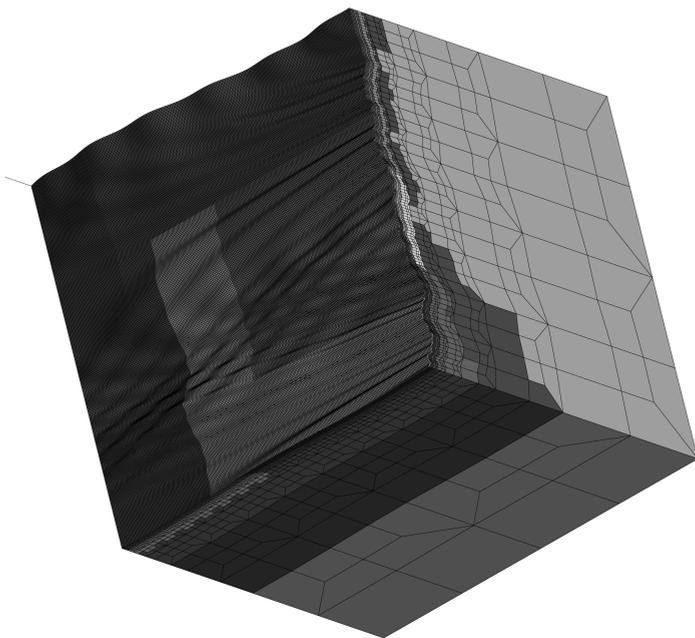
**Fig. 14** The split of the FE mesh split into 16 sub-domains for parallel computations.
