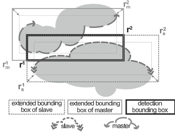
**Fig. 2** Determination of the bounding box for the contact detection procedure in case of simple master-slave contact.
