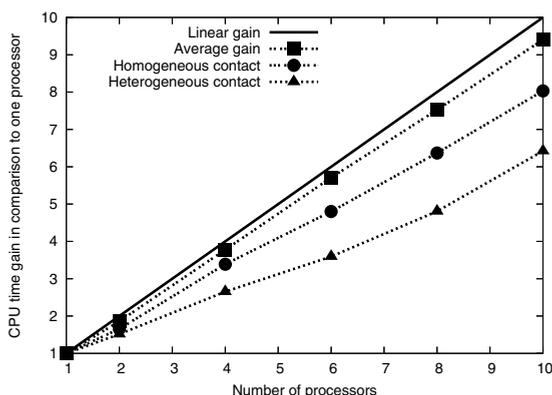
Fig. 15 Time gain for parallel contact detection procedure.
