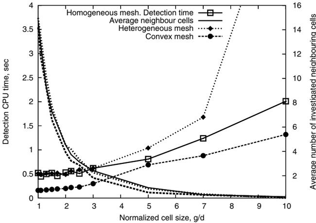
**Fig. 4** The dependence of the detection time and the average number of neighbouring cell investigated during the detection on the normalized cell size.
