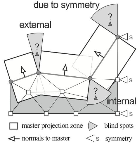
**Fig. 6** Examples of blind spots: external, internal and due to the symmetry boundary conditions.
