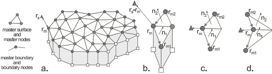
**Fig. 7** Detection of the passing by nodes. (a) Master surface and its boundary. (b) Zoom on the geometry close to the passing by node. (c) Convex master boundary. (D) Concave master boundary.
