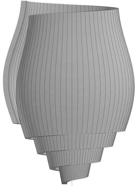
**Fig. 12** Finite element mesh used to test the detection procedure for self-contact problems.
