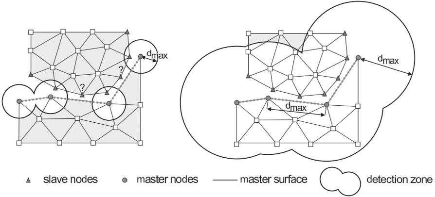
**Fig. 1** Maximal detection distance  $d_{\max}$ : on the left not correct on the right correct choice.
