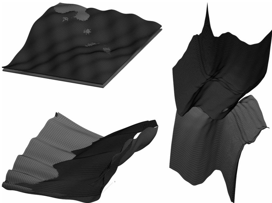
**Fig. 3** Example of finite element meshes used to determine the optimal cell size. Proximal meshes with homogeneous (left top) and heterogeneous (left bottom) spatial node distribution and convex meshes (right).
