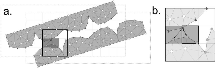
**Fig. 5** Detection of the closest master node in current and neighbouring cell. Slave and master nodes represented by triangles and circles respectively.
