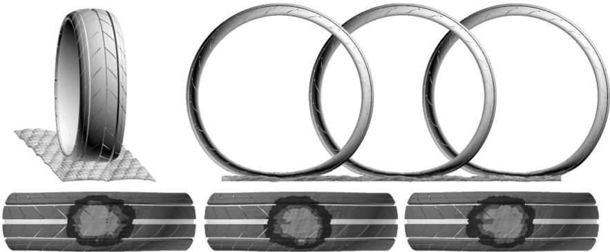
**Fig. 9** Tyre-road contact problem: general view, three tyre-road dispositions and corresponding contact elements on the bottom of the tyre for different imprint deep.
