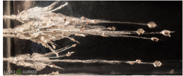
Handgun Self-Defense Ammunition Ballistics Test (bullet penetration in synthetic silicon) www.luckygunner.com
