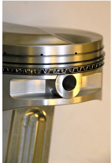
Zoom on grooves and the drain system for oil from www.engine-labs.com
