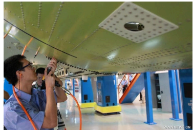
Fuselage of modern aircraft contains \approx 100\,000 rivets
