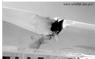
Bird impact traces on aircraft's nose/wing
