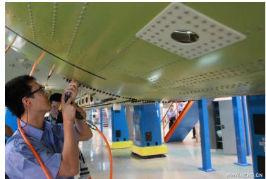
Fuselage of modern aircraft contains \approx 100\,000 rivets
