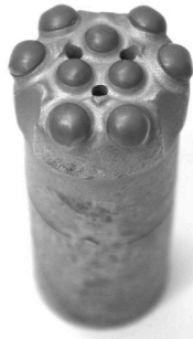
Drill crown and a single drill-bit button WC-Co
