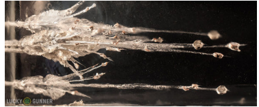
Handgun Self-Defense Ammunition Ballistics Test (bullet penetration in synthetic silicon) www.luckygunner.com
