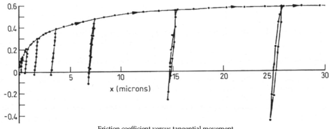
Courtney-Pratt J. S., and E. Eisner. The effect of a tangential force on the contact of metallic bodies. Proc R Soc A 238 (1957)
