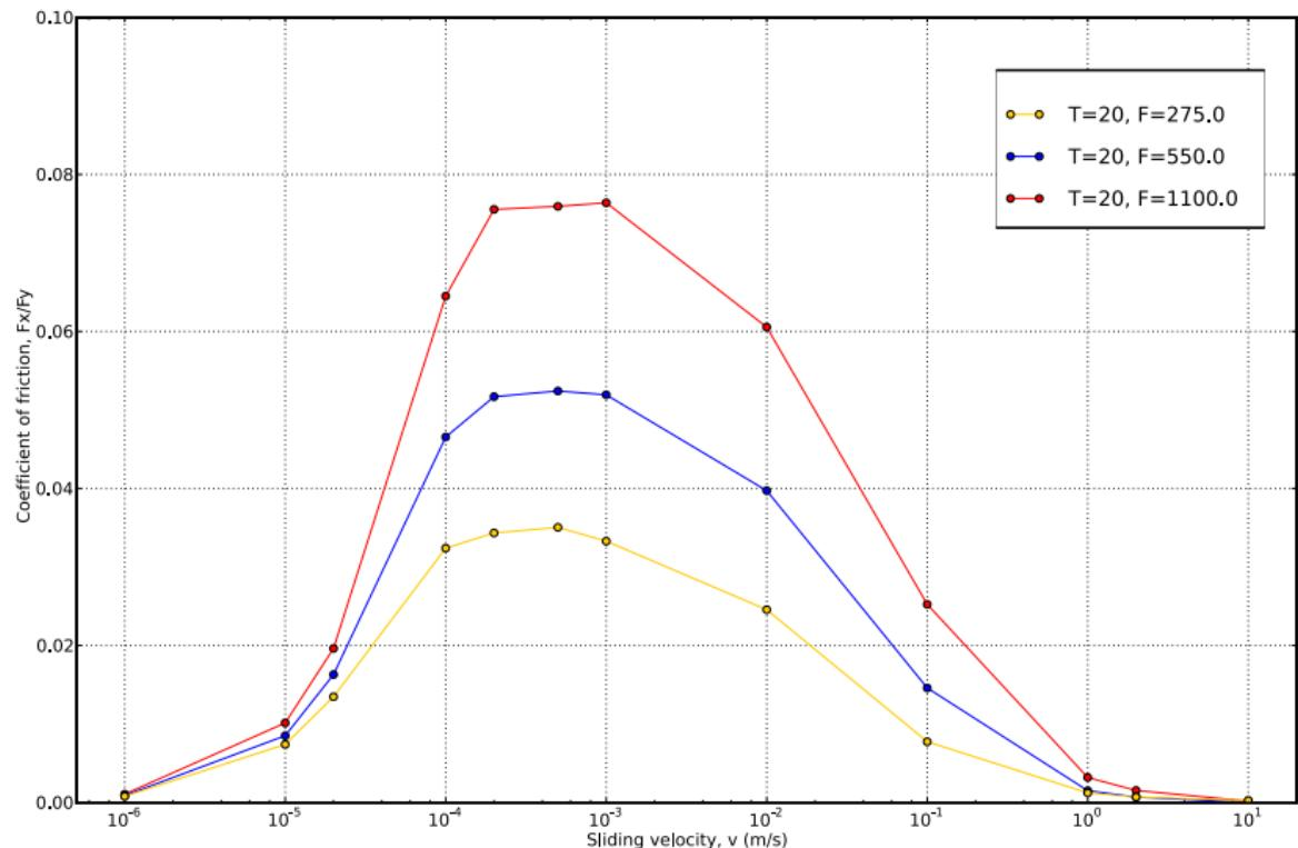
Frictional force at different slip velocity (effect of force)
