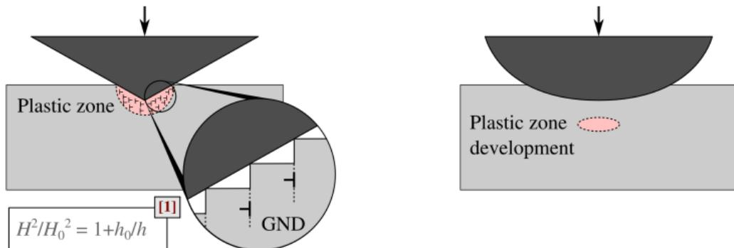
$$\frac{\text{Plastic zone } r}{\text{Contact radius } a} \sim 1 + b \exp(-h/h_1)$$
