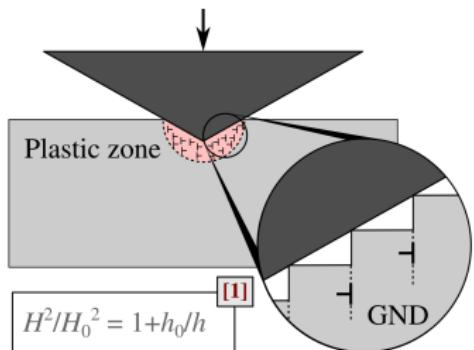
$$\frac{\text{Plastic zone } r}{\text{Contact radius } a} \sim 1 + b \exp(-h/h_1)$$
