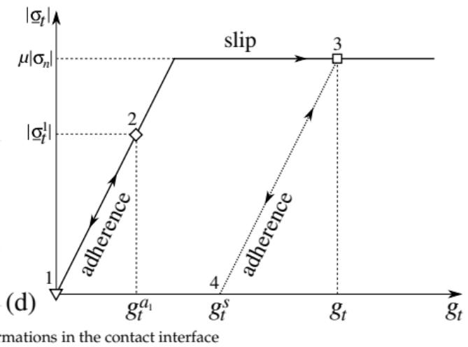
Asperity deformations in the contact interface
