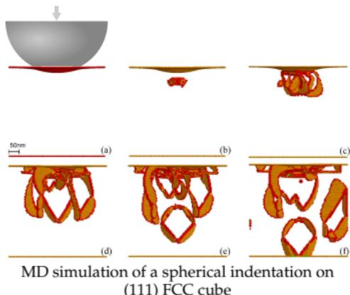
MD simulation of a spherical indentation on (111) FCC cube
