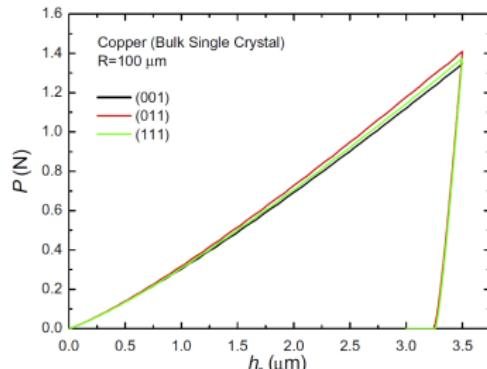
Spherical indentation of FCC copper crystal using crystal plasticity model in Zset
