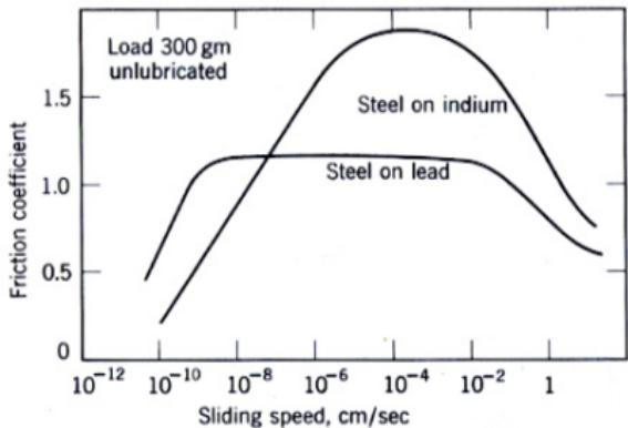
Friction coefficient increases and decreases with increasing velocity of sliding, hard on soft (steel on lead, steel on indium)
