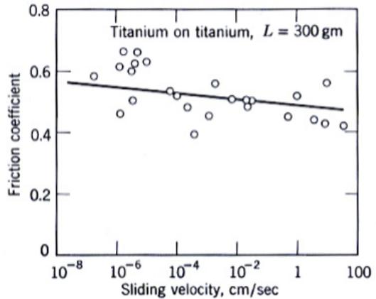
Friction coefficient slightly decreases with increasing velocity of sliding, titanium on titanium
