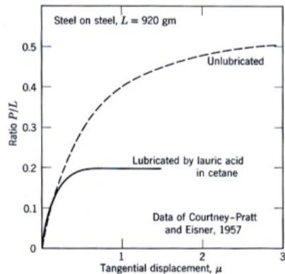
Fig. 1. For very small sliding, the force of friction is not proportional to the normal force<sup>[1]</sup>
