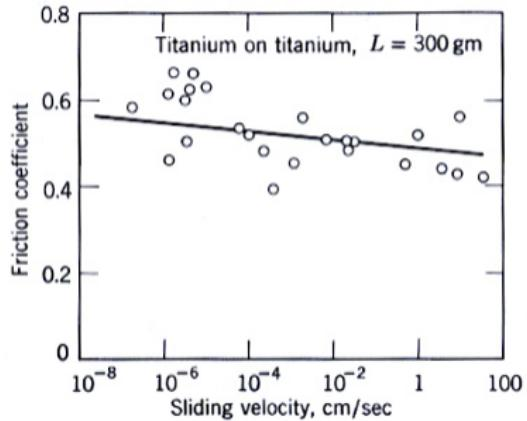
Friction coefficient slightly decreases with increasing velocity of sliding, titanium on titanium
