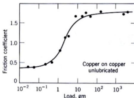
Fig. 2. Hard film on a softer substrate, at moderate loads friction is determined by the film friction, at higher loads, the coating brakes and softer material determines the frictional properties<sup>[1]</sup>
