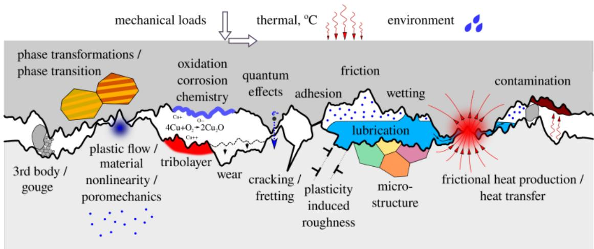
Tribological properties stem from this complex multi-scale physics of interfaces and near-surface layers<sup>[1]</sup>
