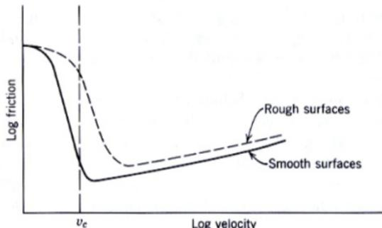
Friction coefficient dependence on velocity of sliding for lubricated surfaces
