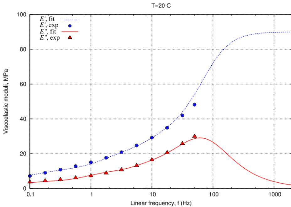
Fitting generalized Maxwell model for rubber to experimental data at
