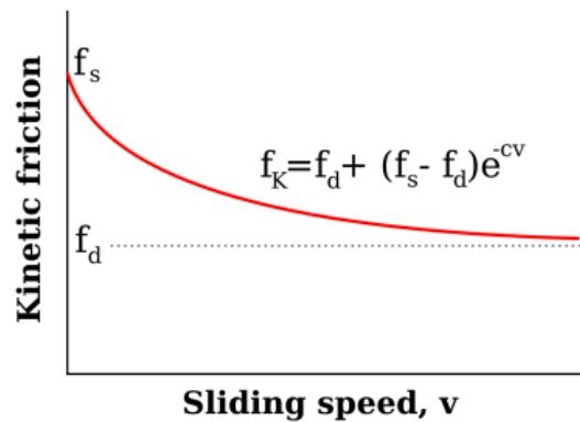
Kinetic friction decreases with increasing sliding velocity
