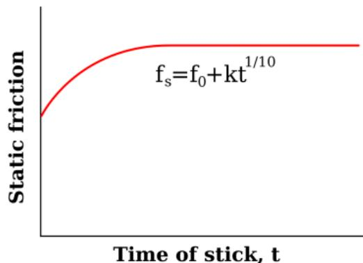
Evolution of the static coefficient of friction with the time of repose
