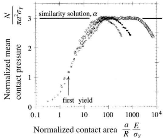
Simulation of spherical indentation of elasto-plastic solid with power-law hardening<sup>[2]</sup>
