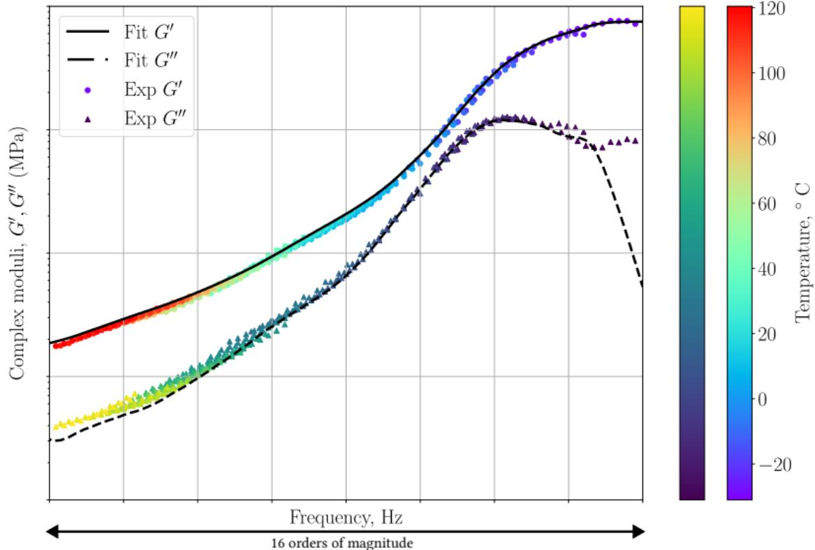
Full data on complex moduli of a sample charged rubber
