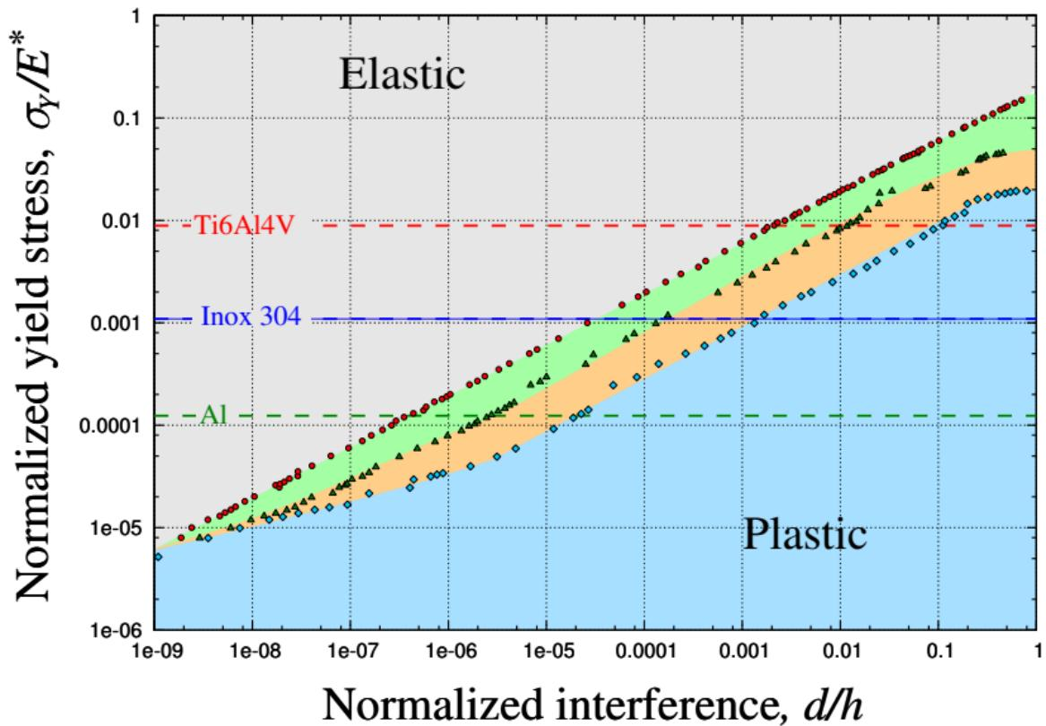
Deformation map for a sinusoidal asperity constructed with M. Liu, H. Proudhon
