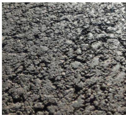
Normal asphalt concrete
