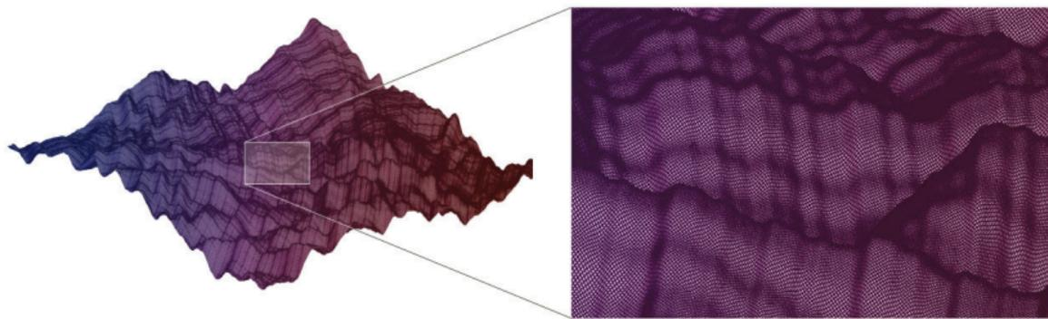
FE mesh of one of the contacting surfaces
