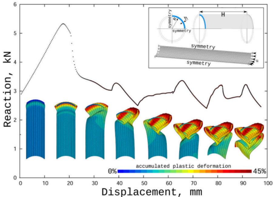
*Finite element analysis of a post-buckling behavior of a thin walled tube*
