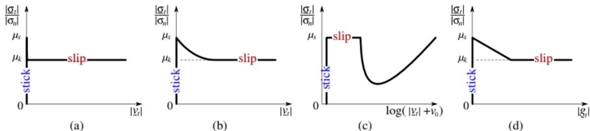
(a,b) velocity weakening    (c) velocity weakening-strengthening
