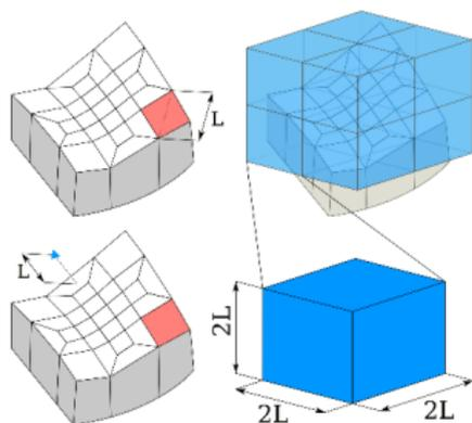
*Relations between the master mesh, maximal detection distance and bucket's dimensions*
