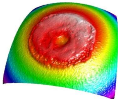
*Damage at electric contact zone*
